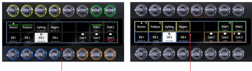
Assign group colors to the LED rings or on the key labels
